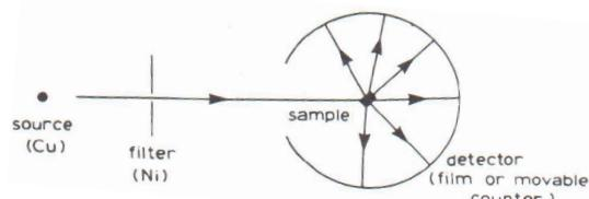
In standard laboratory-based powder diffraction, the data is usually collected by a detector with a slit that is moved along the above circle and it collects data as a function of increasing angle.
