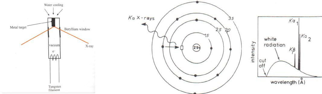
The anode is cooled continuously during x-ray production because not all of the energy is converted into x-rays, much of it is converted into heat and the anode would melt otherwise.
