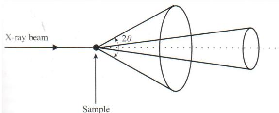
The inner cone has a smaller  $2\theta$  value than the outer cone and hence the inner cone represents a larger  $d$ -spacing. If you have an area detector you can see the circles associated with the diffraction cones.
